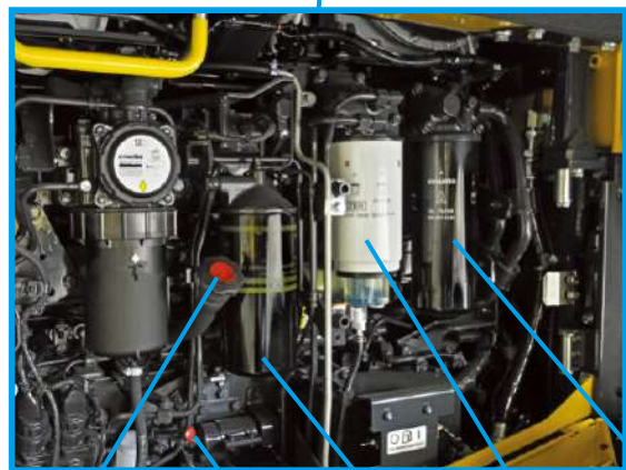
Engine oil fill, Engine oil dipstick, Fuel filter, Fuel pre-filter, Oil filter
