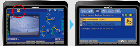
Aftertreatment device regeneration screen
