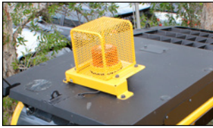
Rotating Amber Beacon Fitted with factory guard.
