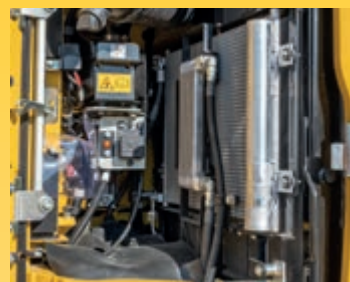
Side-by-side radiator mounting for easy cleaning
