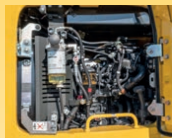
Centralised arrangement of filters
