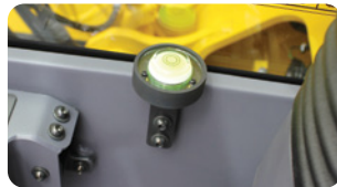
Level Indicator, Overload Alarm & Anti-Burst Valves Enable safety and compliance when lifting suspended loads.
