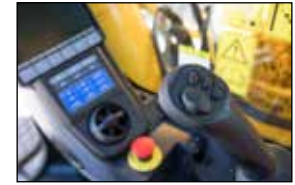
Proportional Hand Controls Enables proportional hand control of attachment speed.
