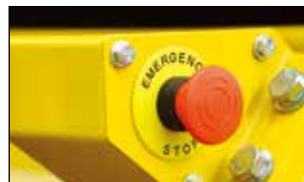
E-Stops Allow compliance to site safety requirements.
