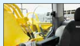
One-touch storable front window lower glass
