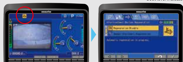
Aftertreatment device regeneration screen
