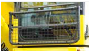
Lower Front Window Guard Protects cabin windscreen against rocks and debris.
