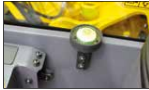
Level Indicator, Overload Alarm & Anti-Burst Valves Enable safety and compliance when lifting suspended loads.
