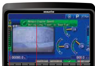
Ecology gauge Fuel consumption gauge Ecology guidance
