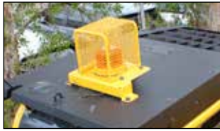
Rotating Amber Beacon Fitted with factory guard.
