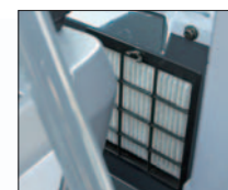
Internal air conditioner filter
